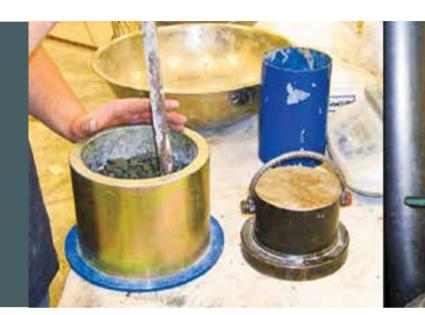
A relative measure of the resistance of an aggregate to crushing under a gradually applied compressive load.
