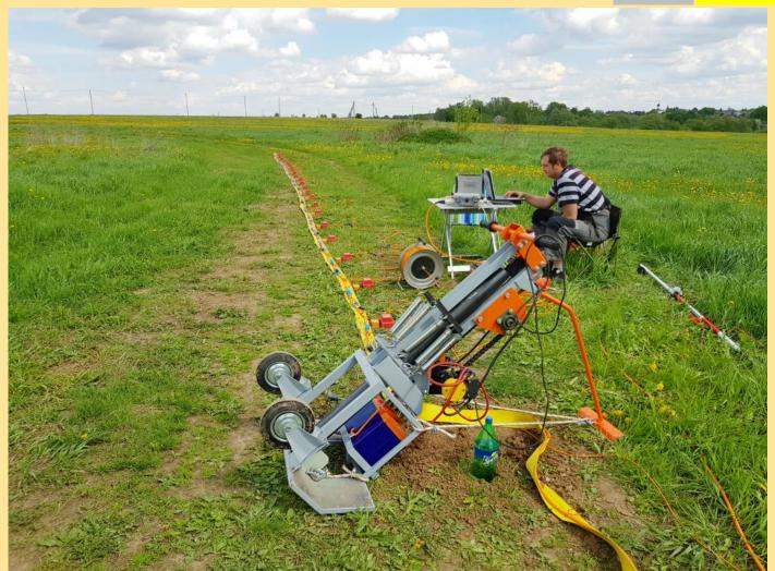
**Vehicle Mounted Accelerated Weight Drop** Seismic Source
